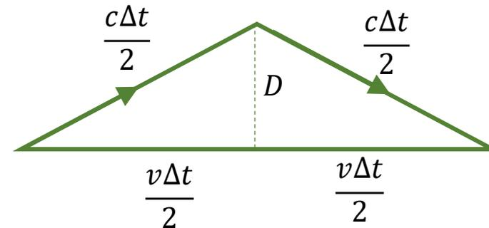
$$\left(\frac{c\Delta t}{2}\right)^2 = \left(\frac{v\Delta t}{2}\right)^2 + D^2 \quad \Rightarrow \quad c^2\Delta t^2 = v^2\Delta t^2 + 2^2D^2$$
